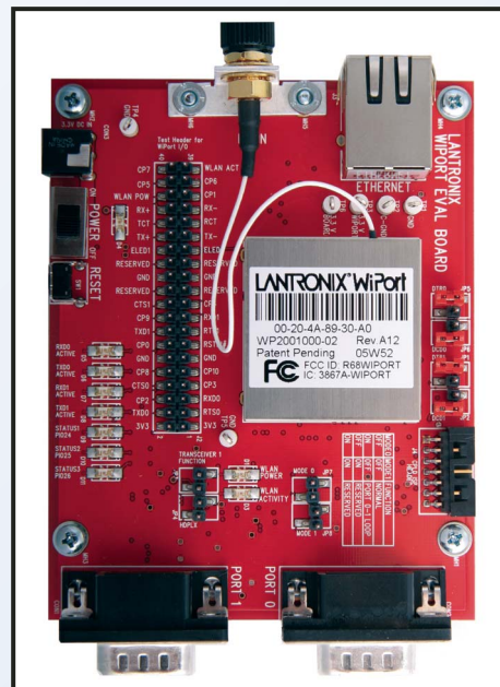
FIGURE 3. Lantronix WiPort evaluation board. The silver WiPort module and pigtail antenna lead are detachable. The 100-gram board (including module) measures 80 x 102 x 17 mm.
