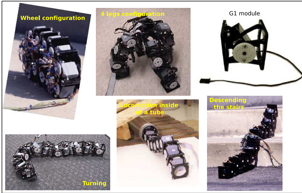
Figure 2.10: Polybot. Different configurations of Polybot G1
