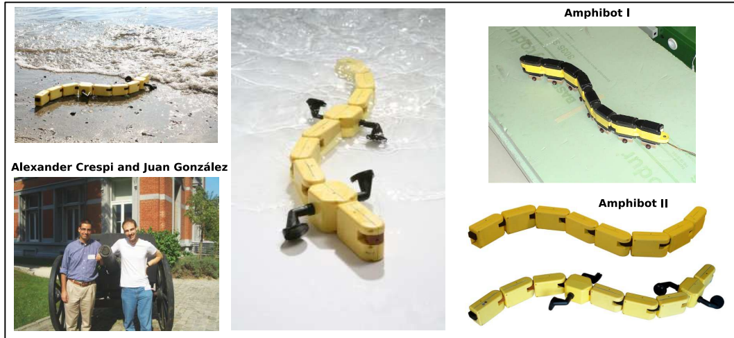
Figure 2.4: The prototypes Amphibot I and II of the EPFL bio-inspired group. The author of this thesis appears at the lower left, together with Alexander Crespi, author of Amphibot, when attending Clawar 2006 in Brussels.
