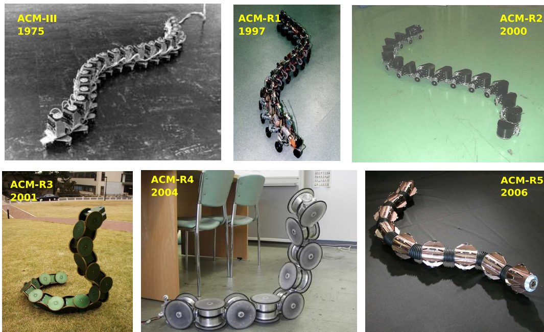
Figure 2.2: Evolution of the snake robots of the ACM family: (Active Cord Mechanism). Hirose-Fukushima Robotics Lab
