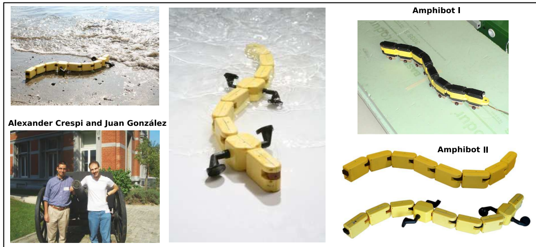
Figure 2.4: The prototypes Amphibot I and II of the EPFL bio-inspired group. The author of this thesis appears at the lower left, together with Alexander Crespi, author of Amphibot, when attending Clawar 2006 in Brussels.
