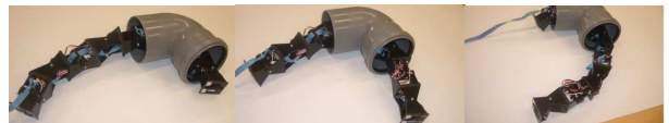
Fig. 16. An example of the turning gait. The robot is going through a curved tube
