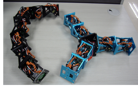
Fig. 8 Snake-like robot and three-leg robot as demonstrators
