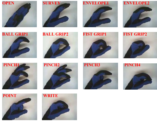
Fig. 6. Hand postures used in the design of the actuator
