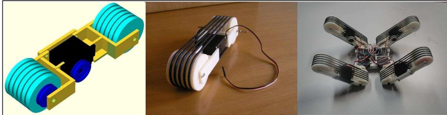
**Fig. 1.9** Unitrack (left) and F-track (right) robots
