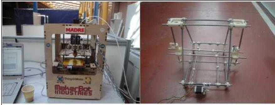
**Fig. 1.3** Our open source 3D printers at Carlos III University of Madrid. On the left: the Makerbot Thing-o-matic, called MADRE. On the right: a Prusa Mendel prototype, being built by the students
